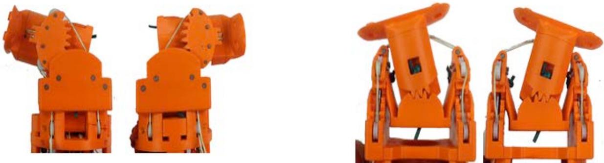
**Figure 3.6** Range of movement of the multidof variable impedance wrist, flexion/extension (right), ulnar/radial (left).
