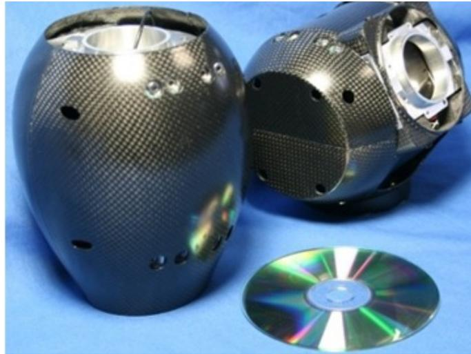
**Figure 4.3** Longitudinal (left) and transverse (right) actuation modules.
