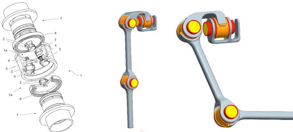
**Figure 3.3** The VSA-Gear Agonist-Antagonist VSA, exploded view and the realization of simple 3D arm with 3 VSA-Gear modules.
