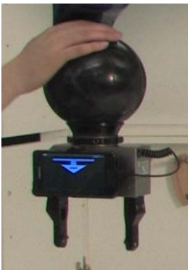
Figure 3: Gripper design used for the SAPHARI human robot interaction experiments. The gripper is based on a Weiss Robotics WSG25 gripper and a Smartphone. This gripper was presented in Milestone 28.
