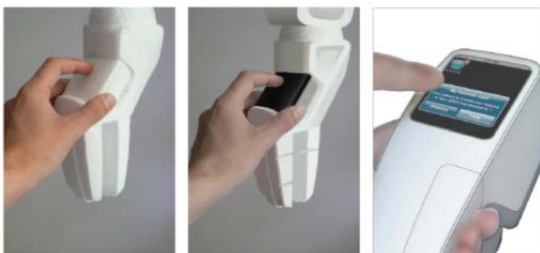
Figure 2: Designer model of gripper for human-robot interaction with touch display
