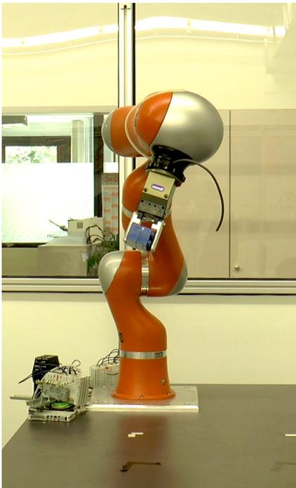
(a) There is a box in the gripper, the tilt is the maximum safe tilt. The robot is stopped by the monitor. The strategy ensures safety.
