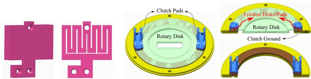
Fig. 8 The L-shape common link of the four-bar mechanisms and the linear drive unit of the variable damping/clutch module
