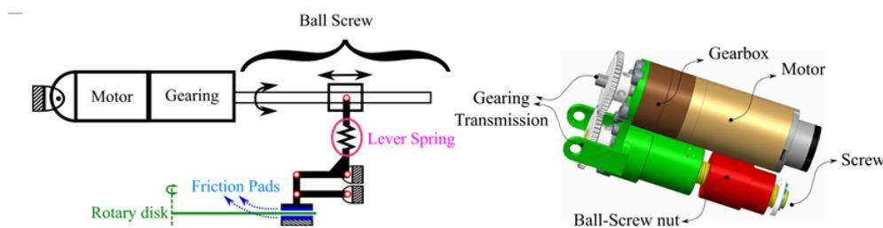
**Fig. 7 Principle and 3D Cad design of the final variable damping mechanism**
