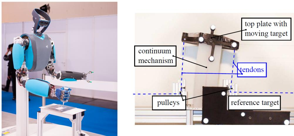
Fig. 11: Left: Full system with two arms and compliant torso; Right: Planar neck prototype
