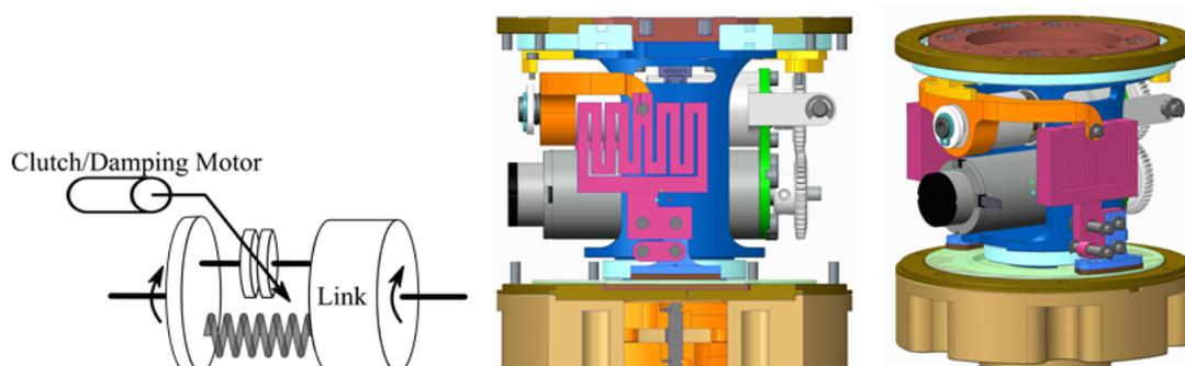
Fig. 9 The overall variable damping/clutch mechanism
