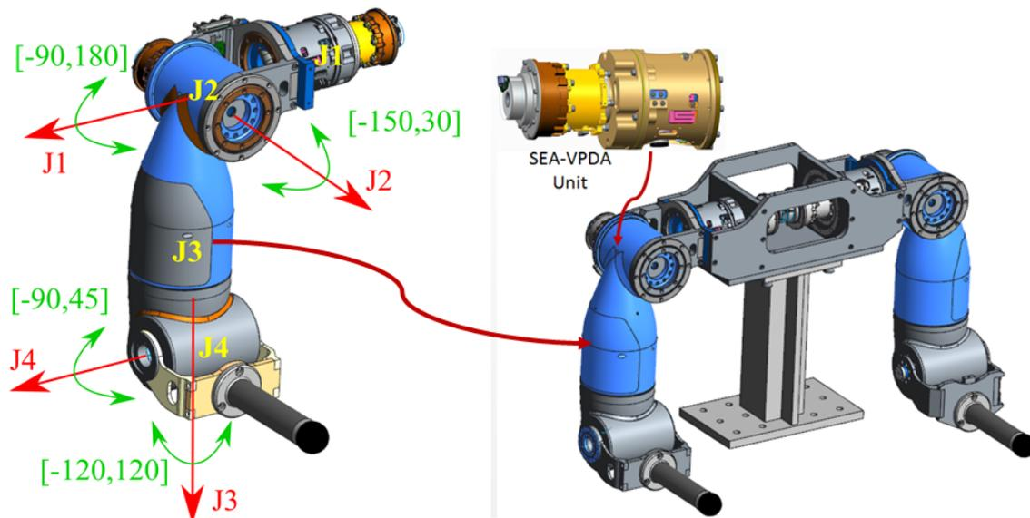
Fig. 5 3D CAD of the the SEA-VPDA dual arm manipulation system
