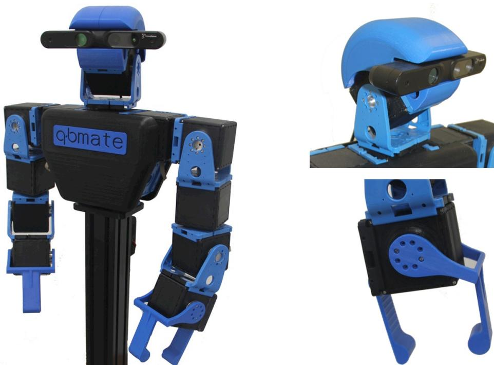
Fig. 2 On the left is shown the complete assembly of the upperbody unit, on the righth some details on the neck and gripper design are highlighted.
