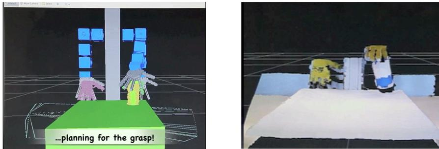
Fig. 3 The execution of the handover task is executed under a ROS and R-VIZ software environment.
