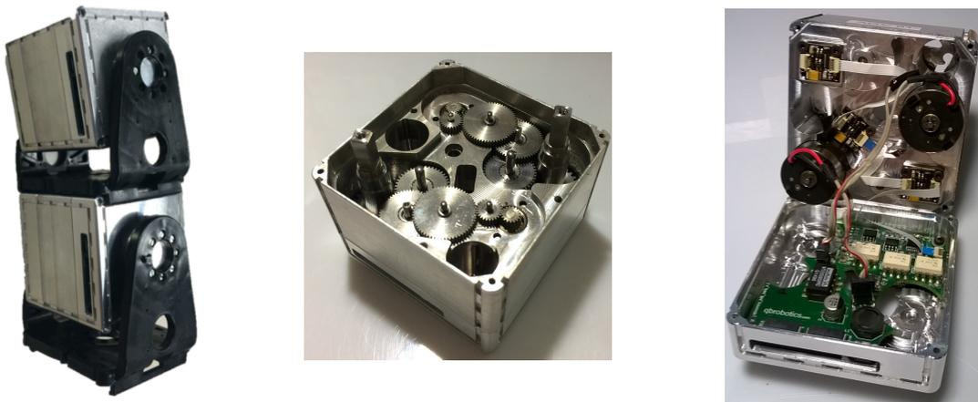
Fig. 1 The picture shows: on the left the external appearance of the *qbmove advanced* together with its compatibility inside the mechanical, electrical and software framework of the platform; on the centre the mechanical implementation of the custom gearboxes and on the right the custom electronic (control, power and sensors) integrated in the mechanical frame of the *qbmove advanced*
