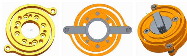
Fig. 6 Compliance system composed of two spiral springs implemented in parallel
