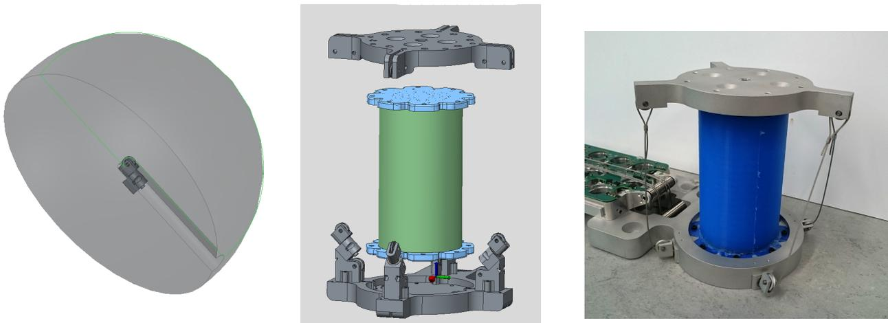
Fig. 12: Left: Workspace of the pulley; Middle: Changeable elastic spine; Right: Final setup
