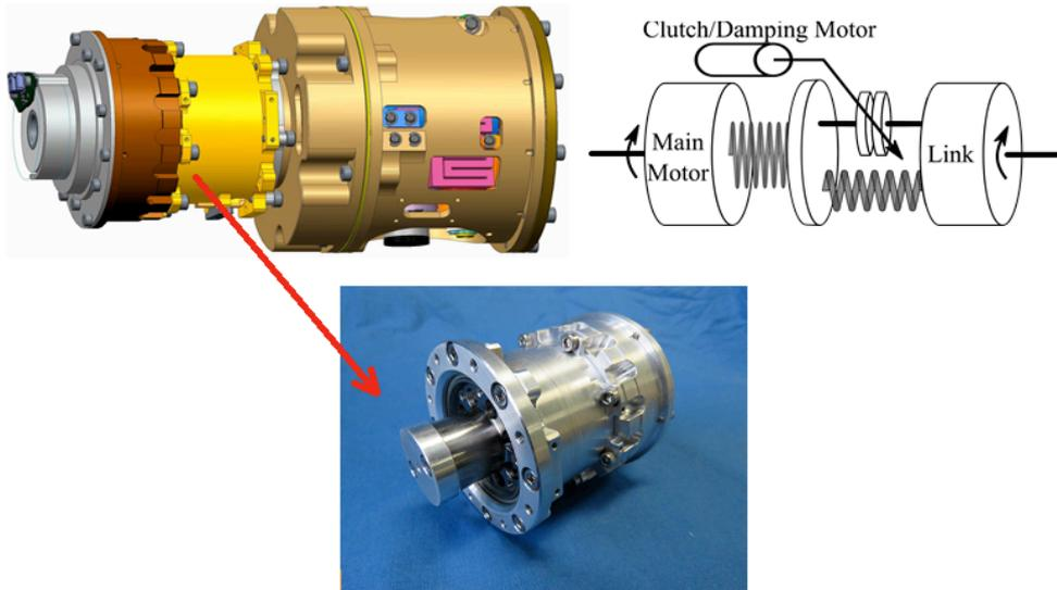
Fig. 10 The complete variable damping/clutch compliant actuation drive
