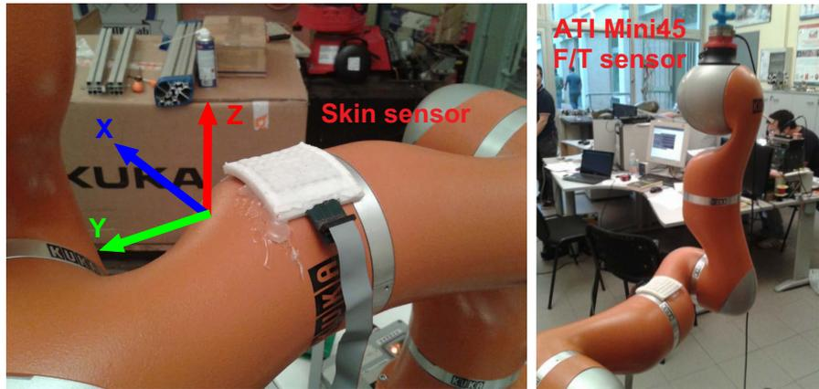
Figure 8: The skin sensor installed on the 3rd link of the KUKA LWR4 robot.
