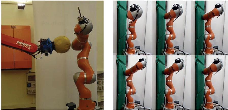
Figure 6: [Left] An elastic ball in interaction with the KUKA LWR4 arm during the first set of experiments. [Right] Snapshot of the KUKA LWR4 robot in contact with a wall during the second set of experiments.
