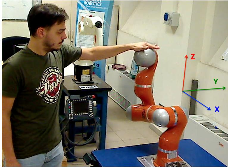
Figure 11: The set-up and the Cartesian reference frame for the contact impedance control experiments. The colors of  $X$ ,  $Y$ , and  $Z$  axes are the same used for the associated components in the plots of Fig. 12.
