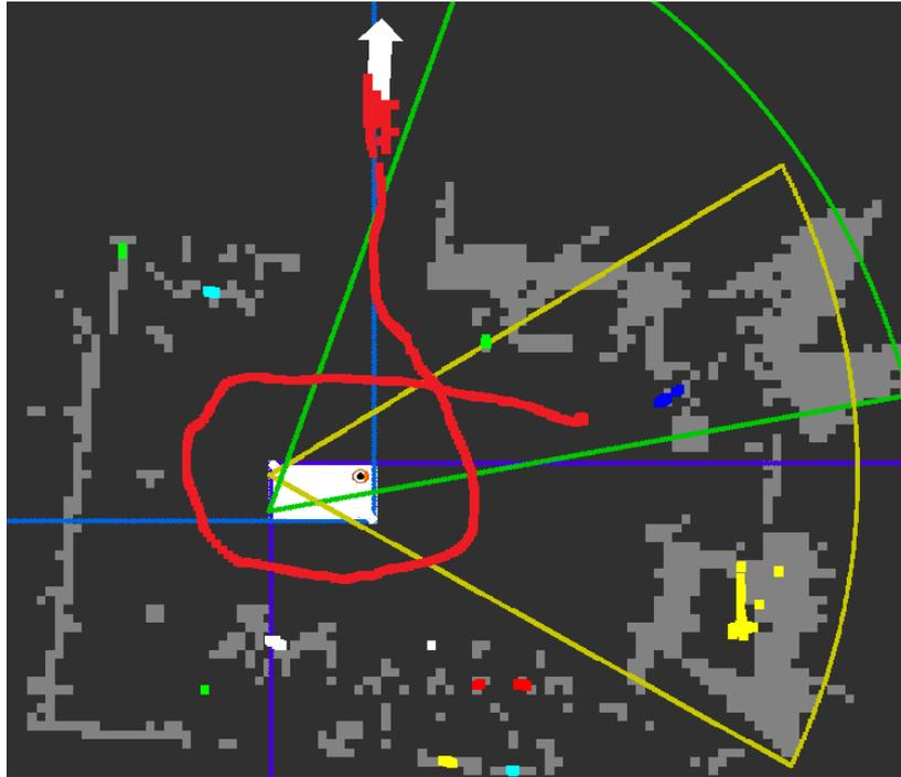
Figure 6: Tracking of a person walking all around the robot.
