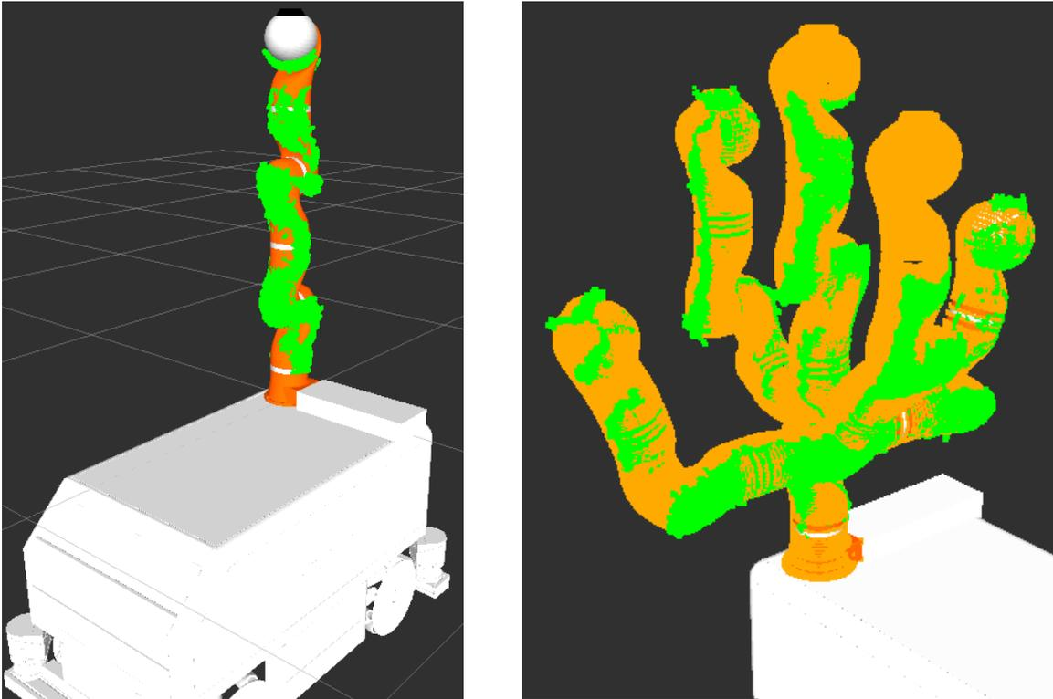
**Figure 2:** Sensor calibration using the manipulator as a calibration target. The point cloud acquired by the 3D depth camera is depicted in green, while the reference point cloud extracted from the model is shown in orange. *Left:* Calibration using a single manipulator pose. *Right:* Point clouds aggregated from a sequence of five poses and fitted by the GICP algorithm.
