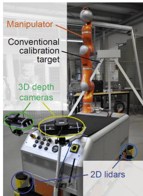
Figure 1: Placement of depth sensors on the mobile manipulator.
