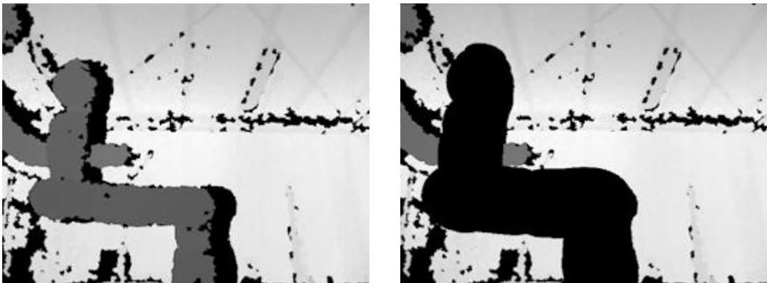
**Figure 3:** Removal of robot points from depth images using the Realtime URDF Filter. *Left:* Acquired depth image of the robot manipulator and a human reaching into the workspace. *Right:* Depth image after removal of the robot points according to the URDF model.
