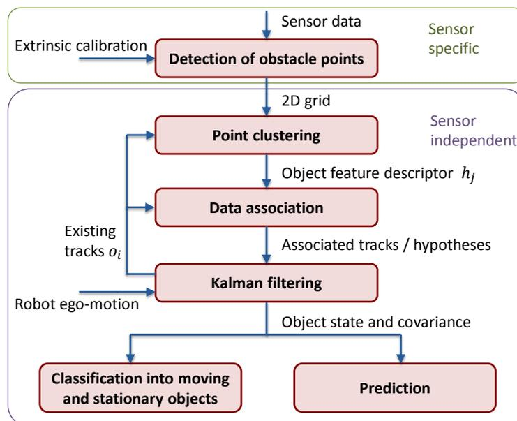
Figure 4: Processing pipeline for obstacle detection and tracking.
