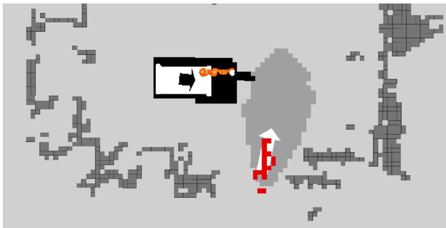
Figure 7: Prediction of human and robot positions for collision prevention.
