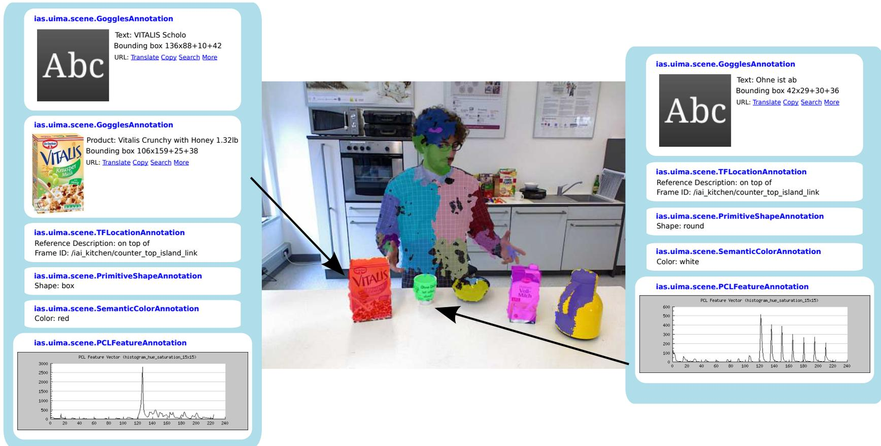
Figure 2: An analysed scene. The original image is overlaid with colored regions representing the recognized objects and bodyparts. The rectangles on the left and right exemplary show annotated properties for two of the recognized objects.
