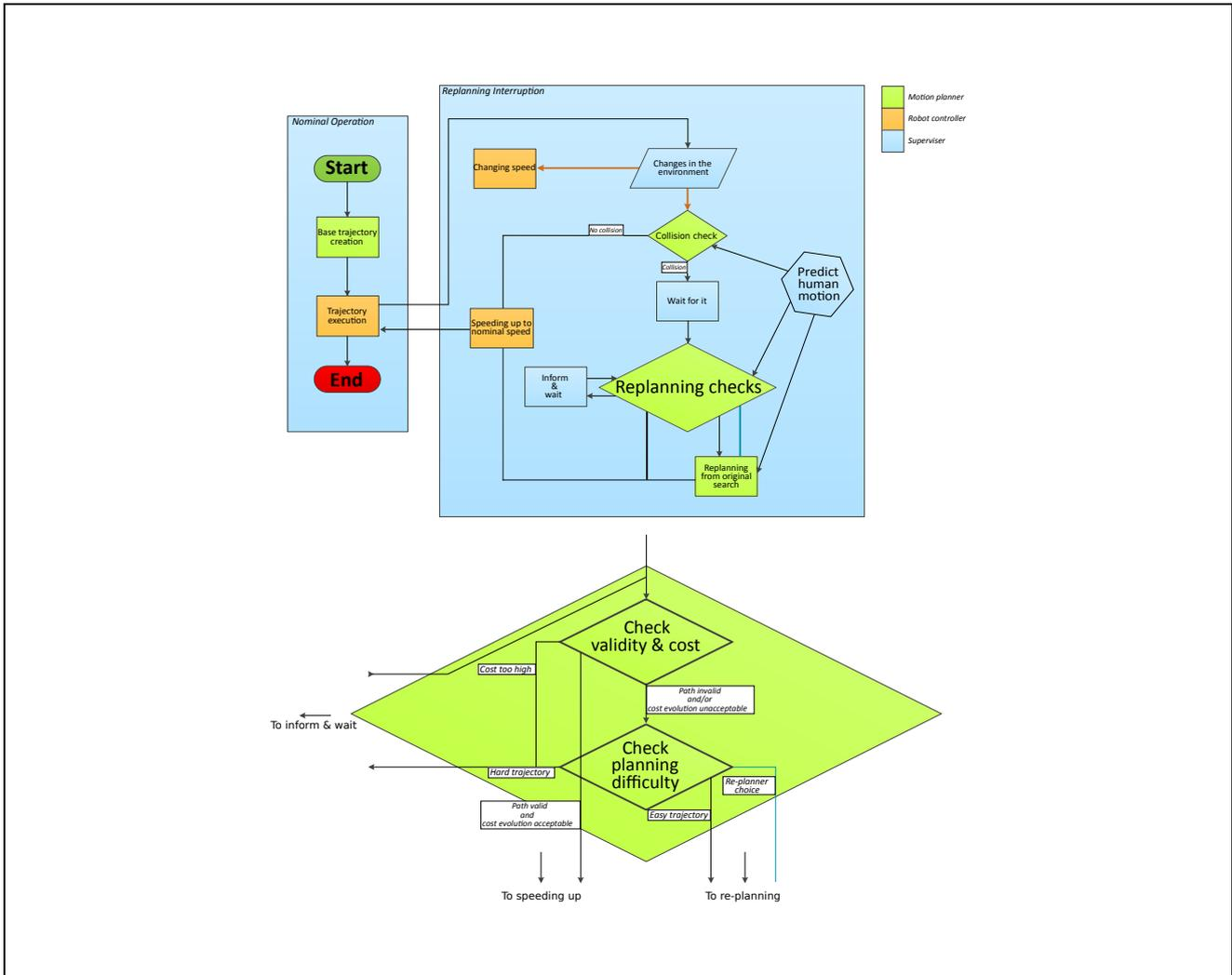
Figure 2: scheme for adapting speed, continuous evaluation of current path and re-planning
