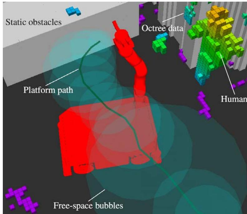
Figure 4: Evasive path of a mobile manipulator computed by the elastic band method.
