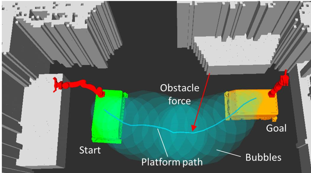
Figure 3: Path adaptation for a mobile manipulator using elastic bands.
