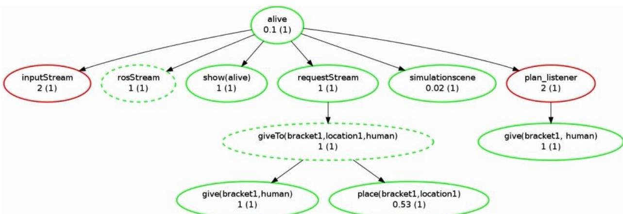
Figure 8: Example of a task tree in the WM: inactive nodes are in red, dotted nodes represent abstract behaviors.
