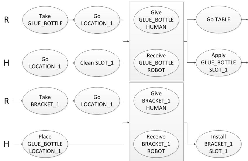
Figure 14: HATP plans: (up) the human is to apply the glue on the SLOT 1; (down) the human is to install the bracket. R and H represent the Robot and the Human actions, respectively; the box highlights the collaborative actions.
