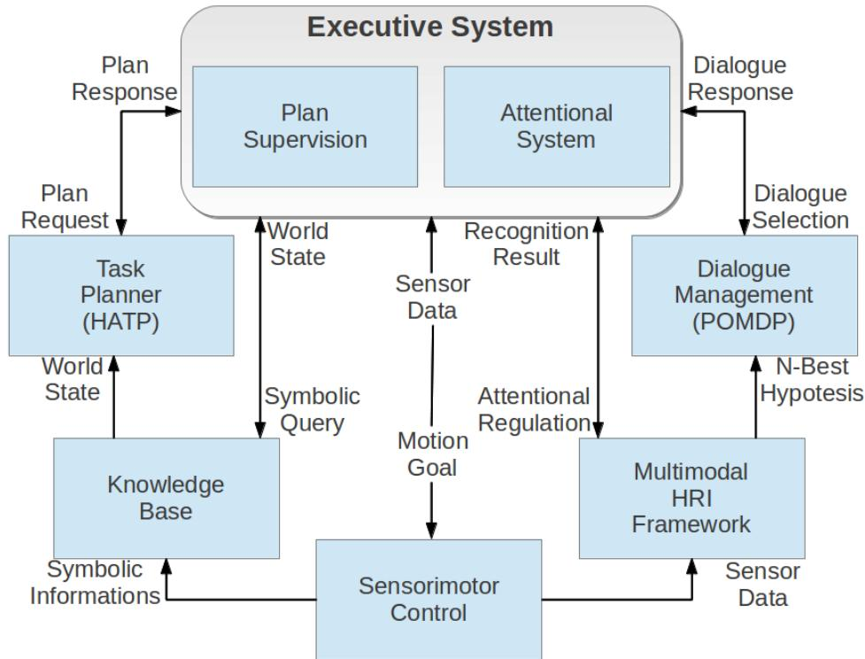
Figure 2: Architecture of the integrated system.
