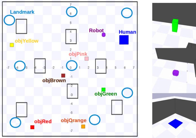
**Figure 4:** Simulated environment: we have colored objects (small cubes), obstacles (black), the human position (large flat square), and the mobile robot (purple).
