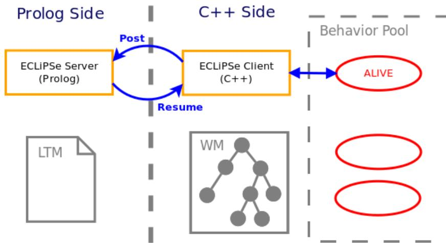
**Figure 11: Sketch of the implemented prototype: the LTM is managed by an ECLiPSe Prolog server; each behavior is implemented by a thread, while a special thread (alive) manages the WM updates.**
