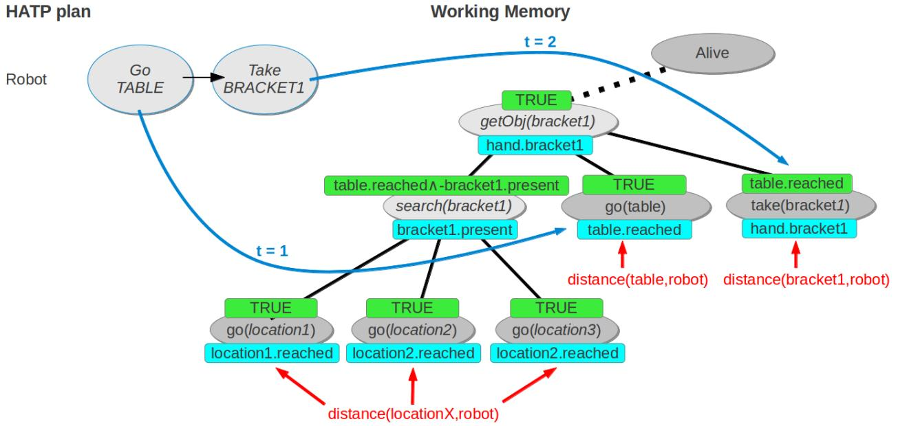
Figure 9: Plan-based (top-down) and environmental influence (bottom-up) during the execution. Green and light blue solids are, respectively, preconditions and goals of tasks/schemata. Top-down regulations are provided by the actions of the HATP plan (blue arrows), while bottom-up regulations are induced by environmental stimuli (red arrows).
